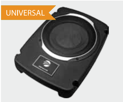
Intelli Sub 10 AFE 250 mm active subwoofer enclosure with the High Level In and Auto-On / Off functionality Frequency range (-3dB): 25 Hz - 100 Hz Active Crossover Low Pass 50 Hz - 100 Hz continuously variable Output power effectively: 100 Watt Maximum output power: 160 Watt Dimensions (WxHxD): 275 x 82 x 369 mm Features: - Very flat - Fits under the driver's seat - Firm die-cast aluminum housing - Dual voice coil woofer with 2 x 2 Ohm - Remote control Part.-No.: 231629 UVP: 299,00 €
