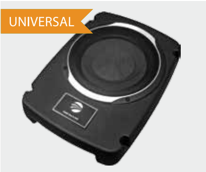
Intelli Sub 8 AFE 200 mm active subwoofer enclosure with the High Level In and Auto-On / Off functionality Frequency range (-3dB): 25 Hz - 100 Hz Active Crossover Low Pass 50 Hz - 100 Hz continuously variable Output power effectively: 100 Watt Maximum output power: 160 Watt Dimensions (WxHxD): 240 x 74 x 345 mm Features: - Very flat - Fits under the driver's seat - Firm die-cast aluminum housing - Dual voice coil woofer with 2 x 2 Ohm - Remote control Part.-No.: 231621 UVP: 249,00 €
