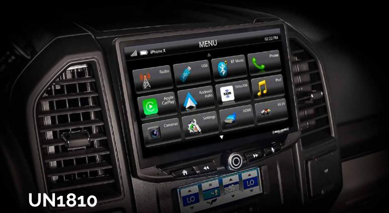
Stinger's radio platform is designed for modular installation, meaning the display and receiver are two separate pieces. This makes it universal for any vehicle, even where space is limited or nonexistent behind the OEM radio being replaced. You can mount the display and reciever in two different locations, giving you flexibility to install HEIGH10® in any vehicle with a standard single or double DIN dash kit. (optional SE-DIN needed for single DIN installations)
