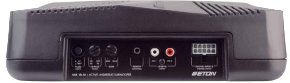
Power, switch-on signal and high-level signal come via the Molex connector; for the low-level there are RCA sockets
