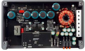
Large sized power supply units, lots of electrolytic capacitor buffers, encapsulated filter coils—the design of the MA amps promises a lot of power just by the appearance
